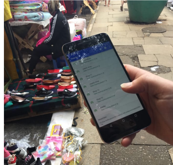
Figure 4: Multiple beacons in range within a shopping district in downtown Nairobi. Selecting any of these will take the user to the simple website of that vendor.
