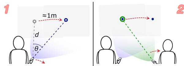
**Figure 3.** Estimating projection surface distance: First, one person calibrates their device by estimating 1m on the projection surface (left). Others calibrate by pointing to markers projected by the first (right).
