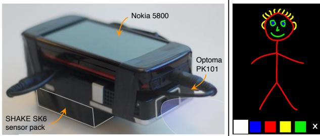
**Figure 2.** Our current prototype. Each user holds the device (left) in-hand, sketching on the screen (right) and moving to animate their projected story. Movements are recorded by the attached sensor pack.
