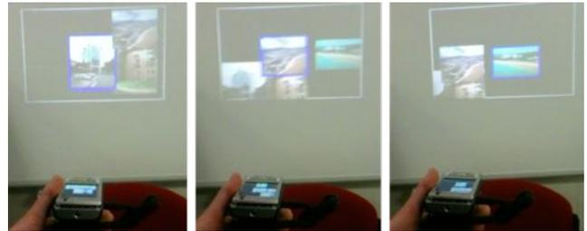
**Figure 2: The prototype in use, showing a user selecting content (highlighted in blue) by pointing the device itself. Content remains stationary to allow easy selection of individual items.**
