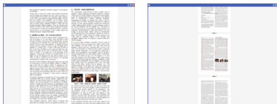
Fig. 1. Document display with traditional (left) and SDAZ (right) scrolling. In SDAZ, the view has shrunk the text and content, providing a less detailed but broader view.
