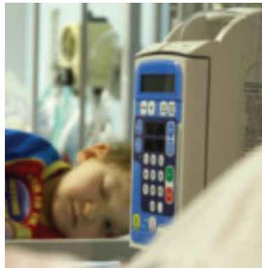
Our research shows numeric keypads (shown) are more error-prone than up/down number entry keys
