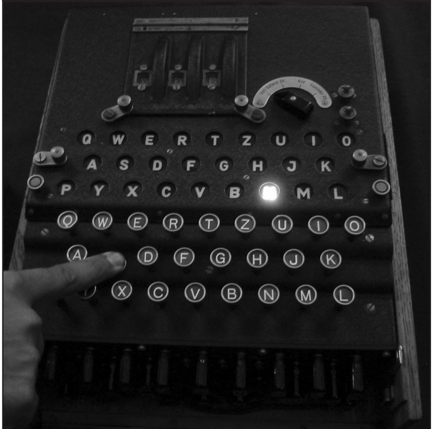
Figure 1. A German army Enigma in use. Here, pressing S lights up N. The three rotors are just visible under the cover at the top; the plug board is partly covered at the bottom.
