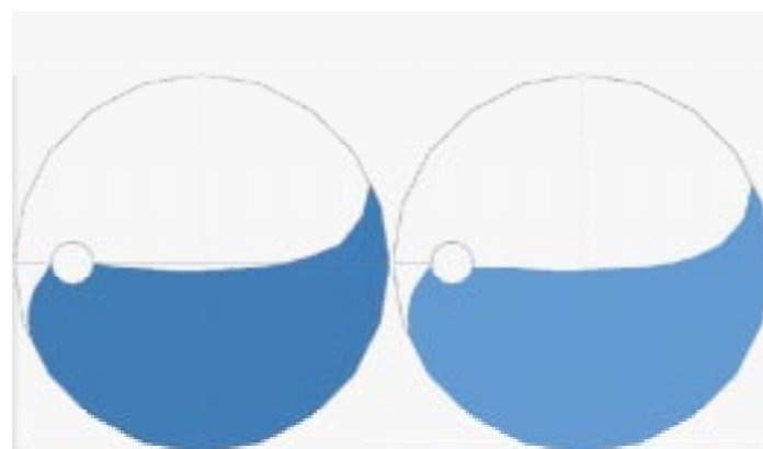
Figure 12. Steady-state surface patterns, twenty rotations (in time), simulations, Re = 8 (50 rpm): left, \alpha_{\text{stir}}=2 ; right, \alpha_{\text{stir-outer}}=1.3 , \alpha_{\text{stir-inner}}=0.8 .
